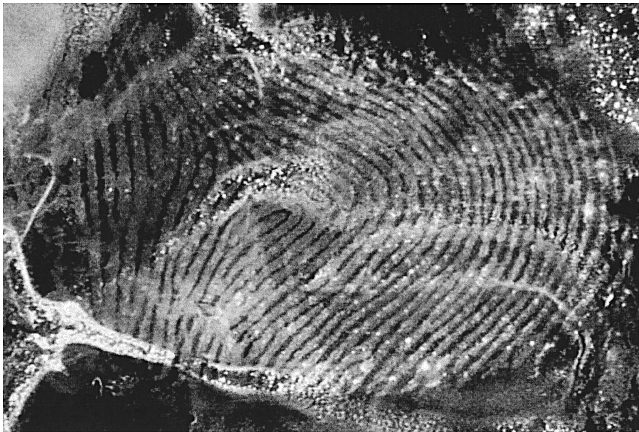
FIG. 2—Cyanoacrylate ester-fumed fingerprint on aluminum foil, developed with CdS/dendrimer nanocomposite in methanol solution.
